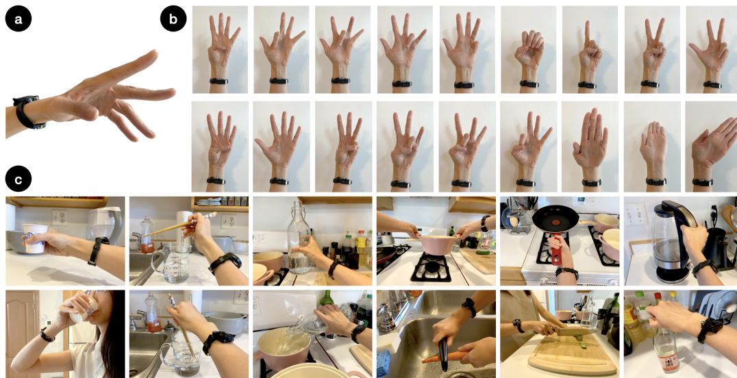
Figure 1: EchoWrist is a wristband that can understand 3D hand pose as well as hand object interactions. (a) The EchoWrist device. EchoWrist adopts a minimally-obtrusive design that keeps the device compact and low-profile. EchoWrist is able to (b) continuously track hand poses and (c) recognize various hand-object interactions.
