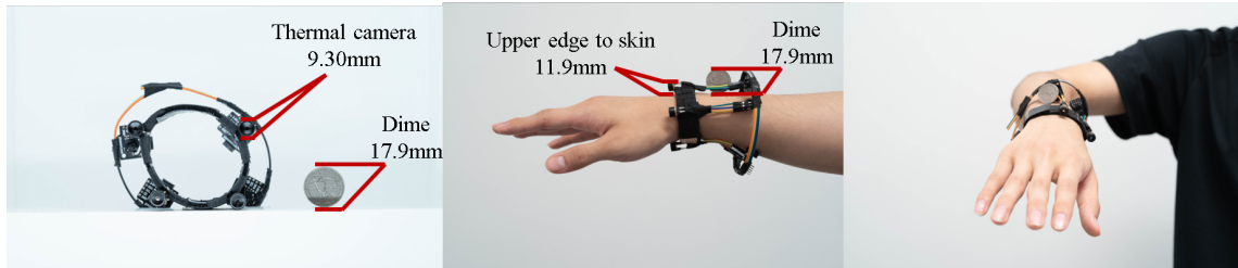
Fig. 5. An illustration of our hardware prototype and its mounting. Left: The prototype wristband sitting on a table and compared to a coin. Middle: The mounting of the same prototype on the wrist and compared to the same coin. Right: A different view of the mounting. We annotate the size of the camera and the coin by millimeter (mm).
