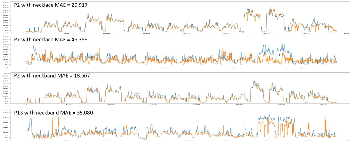
Fig. 12. Ground-truth and prediction blendshape MAE of participants wearing necklace and neckband with highest and lowest performance in sitting scenario without remounting. (Blue line is ground-truth and yellow line is predicted result)
