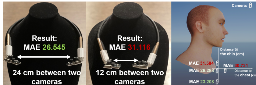
Fig. 11. Camera's position on neckband in pilot study. The result of wider neckband beats the narrow neckband; the lower necklace indicates a better result. 3D mesh model© TurboSquid
