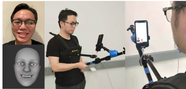
Fig. 6. Left: Camera Captured image and its facial expression reconstruction by ARKit, Left mid: Mobile ground-truth data collection settings, Right mid: User perspective of the mobile settings, Right: iOS data collection application. 3D mesh model© Apple
