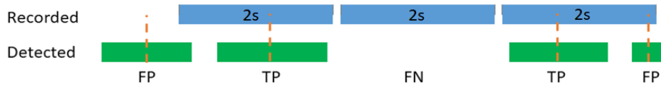
Fig. 6. Evaluation metric for utterance detection. TP: true positives, FP: false positives, FN: false negatives. When the center of a detected segment falls within a recorded segment, it is counted as a TP. If more than one detected segment centers fall within the same recorded segment, only one is counted as TP, other are counted as FP.
