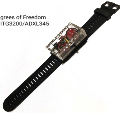
Figure 2: Wristwash device and its integrated sensing capabilities.
